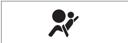
If the "AIR BAG" light on the instrument cluster does not blink or come on when the ignition switch is first turned to the "ON" position, or the "AIR BAG" light stays on, or comes on while driving, the air bag system (or the seat belt pretensioner system) may not work properly. Have the air bag system inspected by an authorized MARUTI SUZUKI dealer as soon as possible.
